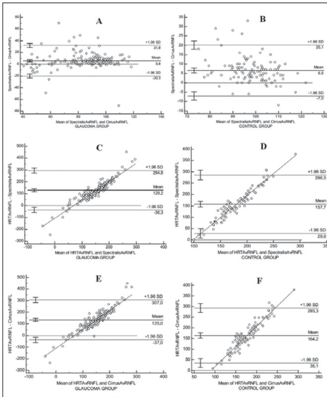
**Figure 1.** Bland-Altman blots indicating agreement of devices for average RNFL thicknesses in glaucoma and control groups. (SpectralisAvRNFL = Spectralis average RNFL thickness, CirrusAvRNFL = Cirrus average RNFL thickness, HRTAvRNFL = HRT average RNFL thickness).
